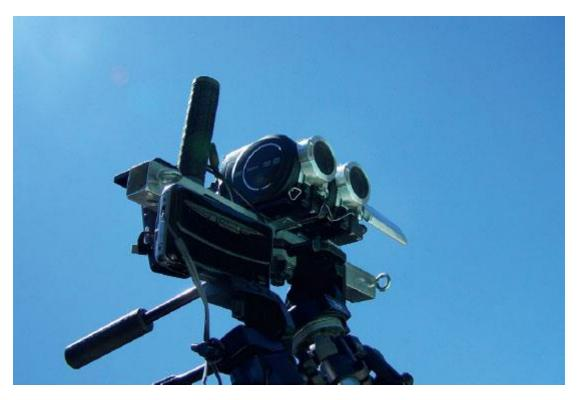
**Figure 23.24** On a single tripod, Razutis has paired two HD cameras side by side with a Fuji W1 3D camera.
