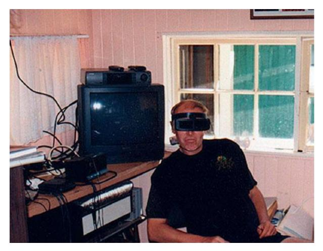
**Figure 23.2** Al Razutis is shown here in 1996 wearing alternating-field liquid-crystal shutter (LCS) glasses for use with his Toshiba 3D camcorder and conventional 60Hz TV.
