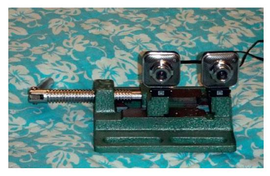
**Figure 23.17** Two CCD sensors in parallel position on one of Razutis's slide bars for 3D capture.
