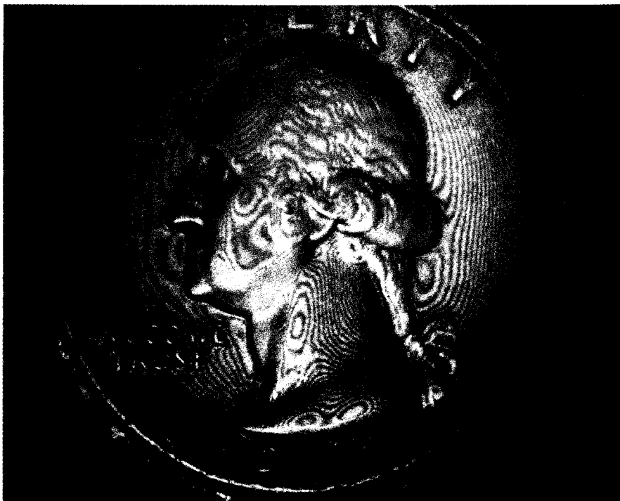
Fig. 25. Holographic Contour Map, made by a method initiated by B. P. Hildebrand and K. A. Haines ( Journal, Optical Society of America , 57, 155, 1967). Improved by J. Varner, University of Michigan, Ann Arbor, 1969.
