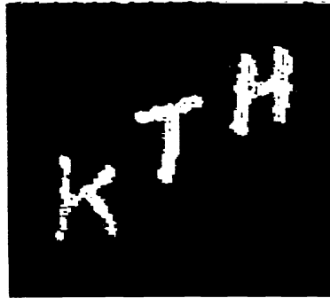
Fig.5. Reconstruction of the letters KTH, where (K) appears at about 35 mm, (T) at 45mm and (H) at 55mm behind the plate. The plate was viewed from the front.
