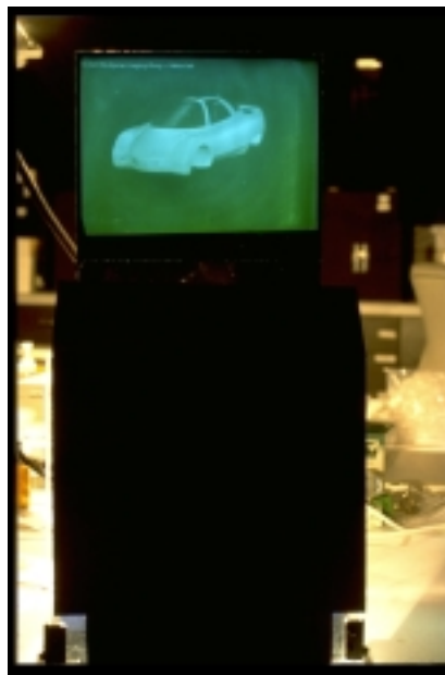
Figure 4: Full parallax image plane holographic stereogram transfer made using the 2X optical magnification. Image size is A4 standard (297mm x 210) and is displayed in a dispersion compensation viewstation.
